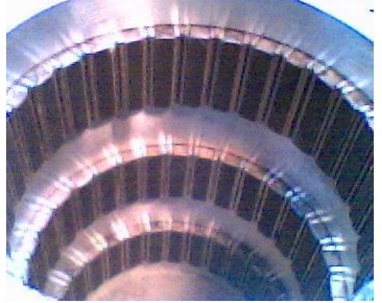
Fig. 15. Inside view of the three-phase rotor.
