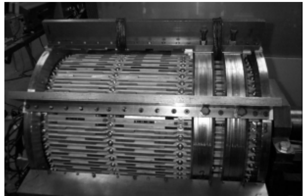
Fig. 11. Prototype of the TFPM machine with toothed rotor. Three stator phases and one rotor phase are shown.
