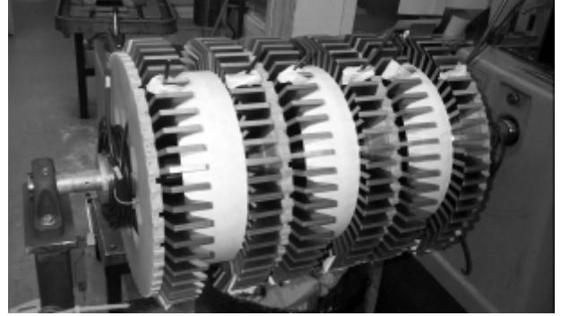
Fig. 10. Stator cores before winding. Rotor and trapeziums not mounted.
