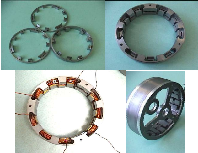
Fig9 Polyphase Claw-pole structure of SMC Brushless PM motor with a centralized-concentrated winding (22 poles)
