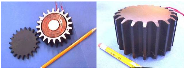
Fig4 SMC Pot-core inductor with "magnetically active" cooling fins
