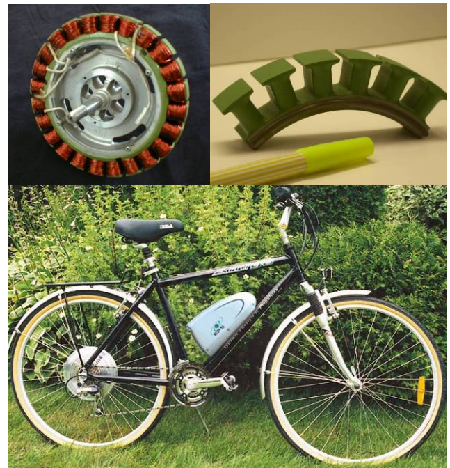
Fig8 Assisted electric bicycle with SMC Brushless PM motor mounted in the rear wheel & realized in 3 sectors
