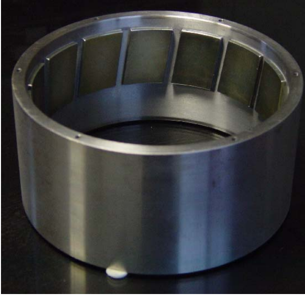
Figure 7. The rotor of the generator with skewed permanent magnets.
